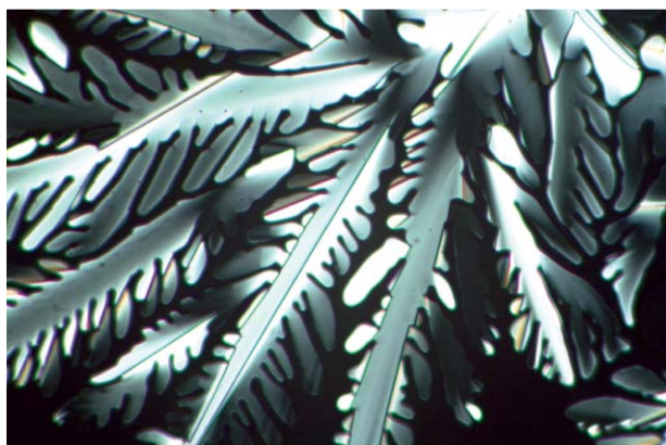
Fig. 2 Optical texture of 3 in the rectangular mesophase.
